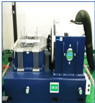
Vibration table x1 10000kgf max force; 2~2500Hz frequency, 2m/s max speed
