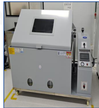
Salt Spray Test device x1 According to ISO 9227:2017
