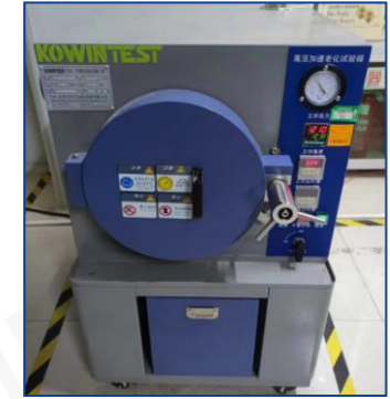
High-pressure boiling testing chamber x1 Temp. range: 100~132°C R.H. range: 100% R.H. Pressure: <5atm
