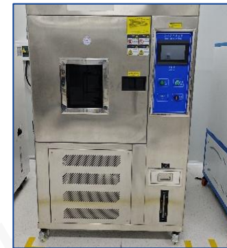
Xenon lamp aging tester x1 According to DIN 75220
